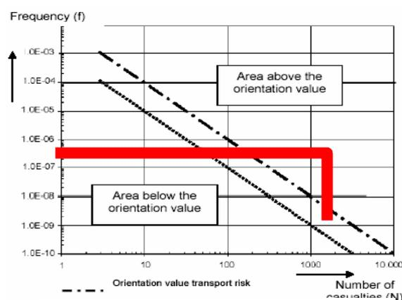
Figure 2: Schematic reproduction of an exceeding of the Group Risk criterion.
