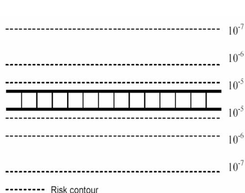
Figure 1: Schematic visualization of Individual Risk near a railroad.
